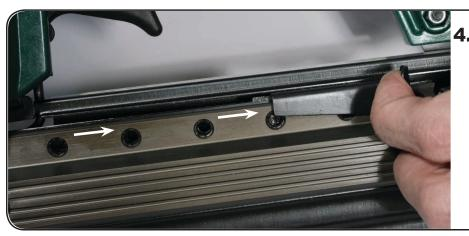
To load nails, remove the air hose from the tool then slide the pusher towards the rear of the magazine. The rail cover will open to the side.
